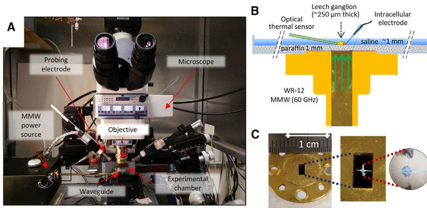
(C) Shown is a photograph of WR-12 waveguide top view (*leftmost picture*) with enlarged picture of its aperture overlapped with a picture of the leech ganglia (*middle picture*) and enlarged photograph of the ganglia (*rightmost picture*) stained with 1% trypan blue, fixed in cold 4% paraformaldehyde and 0.1 M phosphate buffer (pH 7.4), and washed in PBS. The circle indicates the position of one N lateral (NI) thermosensitive nociceptor neuron. To see this figure in color, go online.
