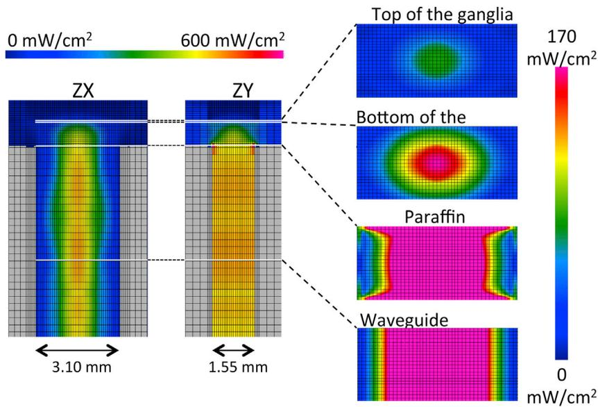
FIGURE 3 Finite difference time domain simulation of the MMW power distribution in the experimental setup. Shown is the power distribution throughout from the waveguide and through chamber in ZX and ZY projections (*left*) and power distribution on the different XY levels of the model (*right*). The power density estimated at the bottom of the ganglia was 170 mW/cm<sup>2</sup> and at the top was 85 mW/cm<sup>2</sup>. To see this figure in color, go online.
