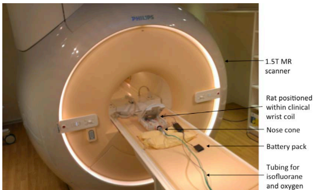
Figure 7.1 The position of the rat within the clinical wrist coil and the 1.5T MR scanner.
